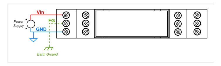
If earth ground is not available FG can be left floating or it can be connected with the power supply GND.
