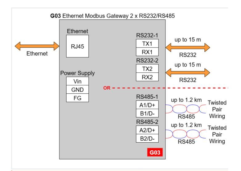
In the G03 gateway user should use only RS232 or only RS485 interface of one port as they occupy the same internal bus of the device.
