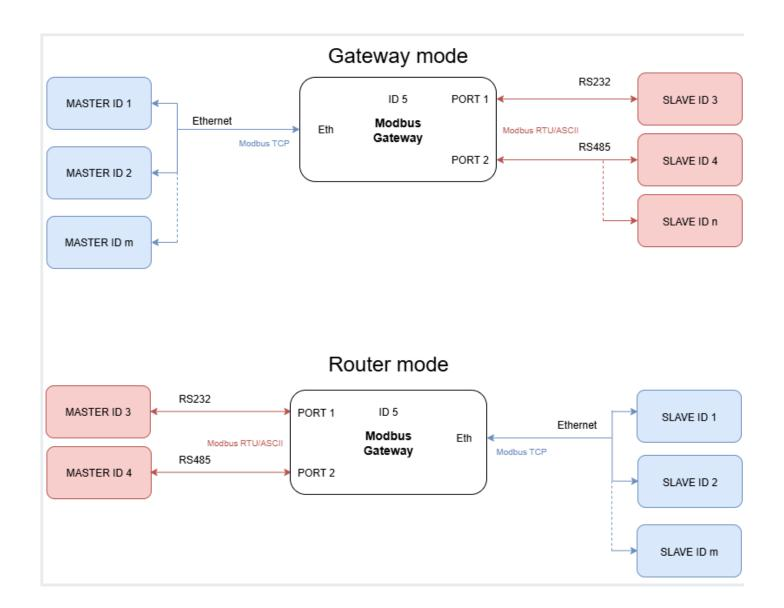
The device has max 20 sockets open in Gateway mode and max 8 in Router mode. It is possible to increase this value at client's request.
